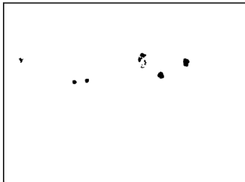
Rust Grade 7-G, 0.3% Rusted
